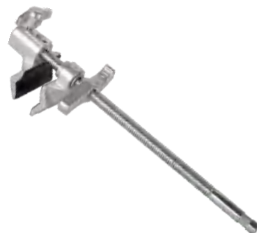
M11-078C 420mm长平夹 End Jaw Clamp with 5/8" Pin & Hex Socket 16-265mm 0.96 25kg
